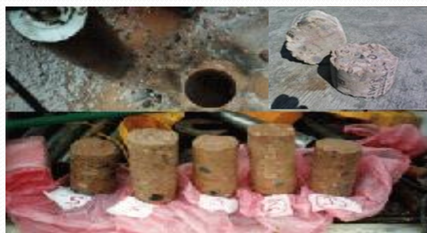
Stabilized Soil/Crushed Stone Samples
